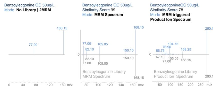
Figure 4. Compared to a conventional 2 MRM data analysis, MRM Spectrum and MRM triggered product ion spectrum data acquisitions deliver library searchable spectra for benzoylcegonine spiked into whole blood at a concentration of 50ug/L.
