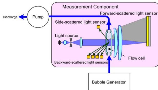
Figure 2: Measurement with Flow Cell Connected to Bubble Generator
