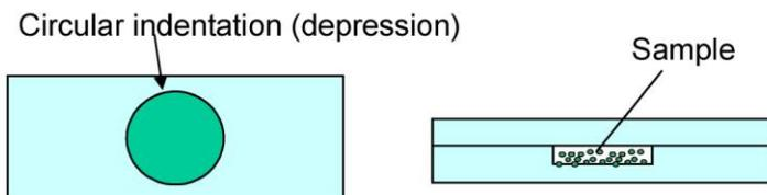
Figure 3: Cell for Extremely Small Bubble Quantities (Crater Cell)
