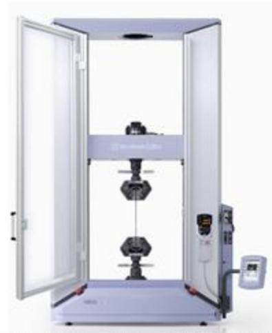
Fig. 1 External View of SHIMADZU Autograph AG-X
