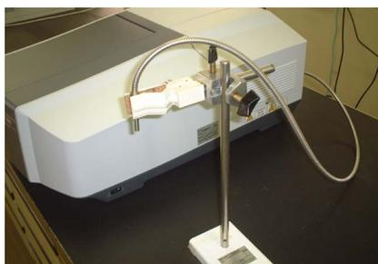
Fig. 1 UV-2600 and Emission Spectrum Measurement Accessory
