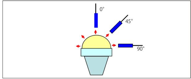
Fig. 7 Comparative Directional Emission Spectrum Measurement
