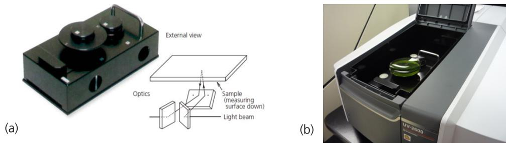
**Figure 2:** (a) 5 degree relative specular reflectance accessory and external view of light beam path with accessory in place; (b) 5 degree relative specular reflectance accessory sitting in UV-2600 sample compartment with acrylic lens in place.
