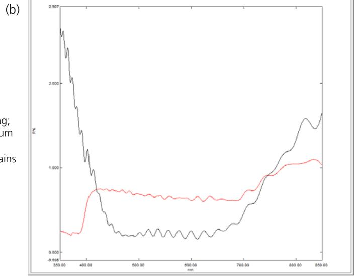
The industry of applying coatings as thin films relies heavily on the ability to determine the thickness of the coating for quality control purposes. In ophthalmics spectral reflectance is used to measure AR as well as hard coating thickness. The ophthalmic industry takes advantage of the capability to add
