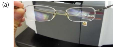
**Figure 1:** (a) Ophthalmic lens with AR coating and hard coating; (b) Reflectance spectra of ophthalmic lenses. The black spectrum represents a lens that contains both a hard coating and AR coating, whereas the red spectrum represents a lens that contains only a hard coating.
