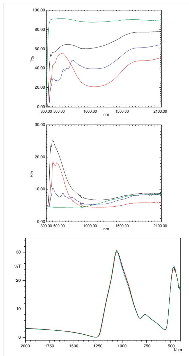
**Fig. 1 Transmission Spectra (upper) and Reflection Spectra (middle) in UV-VIS-NIR Region Reflection Spectra (bottom) in Infrared Region**
