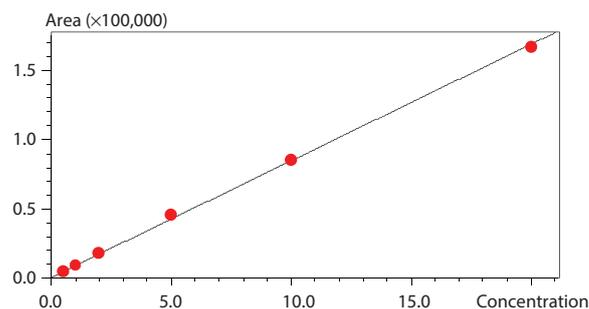
**Fig. 2 Calibration Curve of Bromate (0.0005 mg/L to 0.01 mg/L)**
