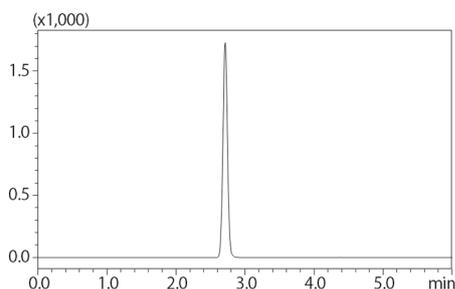
**Fig. 1 Chromatogram of Standard Solution of 0.001 mg/L Bromate**
