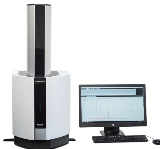
Fig. 1 Benchtop MALDI-TOF MS: MALDI-8020
