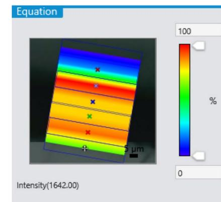
All the different types of analysis can be conveniently edited within the AIMsolution software. These analysis features and the high sensitivity of the liquid nitrogen cooled MCT detector make the AIM-9000 FTIR microscope an ideal tool in the investigation of cross section of polymer films.
