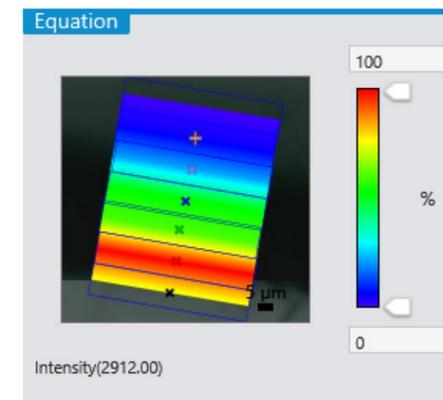
The peak at about 2912  $\text{cm}^{-1}$  was attributed to symmetric and antisymmetric stretching of C-H bond. Since a concentration gradient of  $-\text{CH}_2-$  exists over the cross section, the peak intensity of this IR mode serves as a good indicator of varying chemical compositions. A monotonic change of the peak intensity was observed from one side of the sample to the other (Figure 5). Peak intensity analysis can be applied to other IR modes as well.
