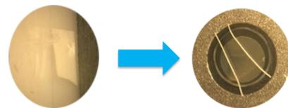
Figure 1. The composite film was loaded onto a microtome and cut into thin slices for cross section studies. The cut slices were loaded onto a diamond window and transferred to the AIM-9000 FTIR microscope
