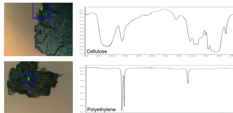
Figure 5. IR spectra of cellulose (top) and PE (bottom).
