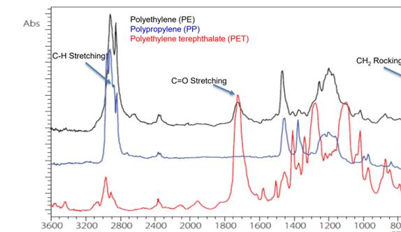
Figure 6. Data obtained from the FTIR systems were matched with library database to identify and quantify microplastics
