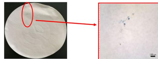
Figure 4. Microplastics on cellulose filter paper
