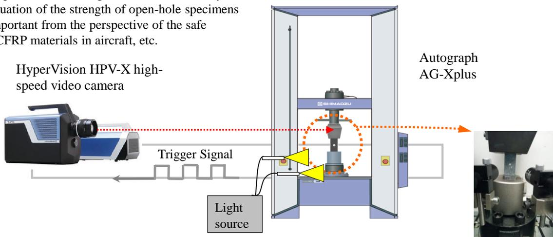
Fig.1: Testing Apparatus
