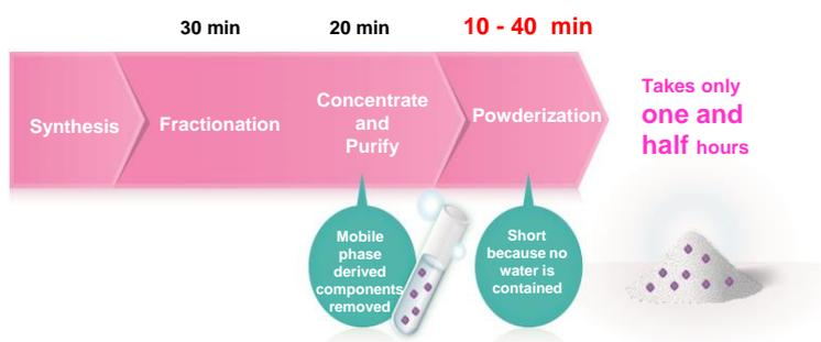
Figure 12. UFPLC purification cycle
