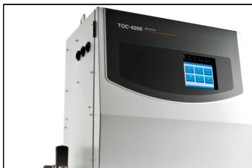
The self-calibration option and an automatic dilution function enable a virtually independent operation of the measuring system which can be started and calibrated from one measuring station. The different measuring streams can be selected.
