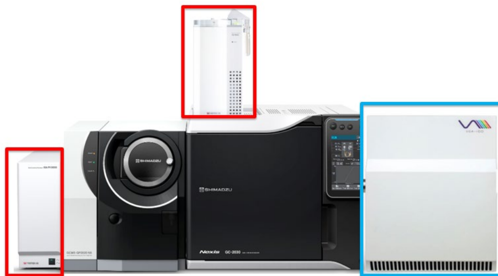
Figure 10: Photo of TD-GCMS-VUV. Center is a Shimadzu Nexis GCMS-2020, on the right in the blue outline box is a VUV detector from VUV Analytics, and on the left and top are the red outline boxes for the Thermal Desorption unit from Frontier Lab.
