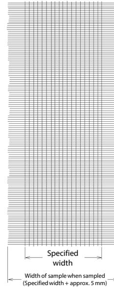
**Fig. 1 Schematic Diagram of Raveled Strip Method Sample**
