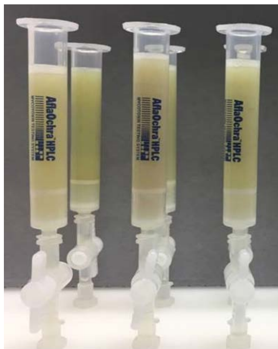
Figure 1: Afla-Ochra Column for extraction/clean-up
