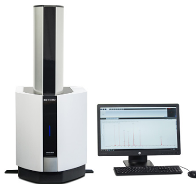
Fig. 1 Appearance of Benchtop MALDI-TOF MS "MALDI-8020"
