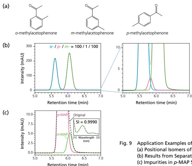
Fig. 9 Application Examples of Peak Separation Algorithm using i-PDeA II
