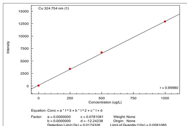
Figure 2: Calibration Curve of Copper
