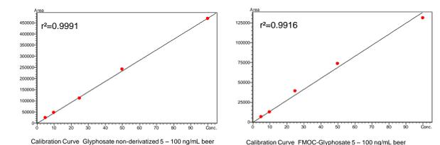
Figure 4: Calibration curves of Glyphosate determined in duplicate obtained from beer after sample pre-treatment. R<sup>2</sup> was better than 0.99.
