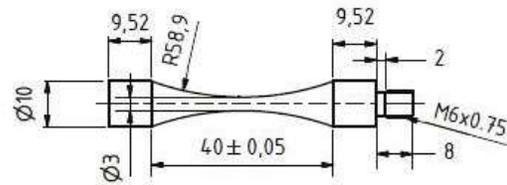
Fig. 3: Specimen geometry for ultrasonic fatigue tests
