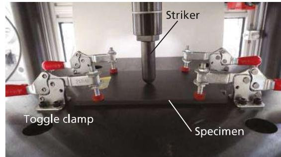
**Fig. 1 Impact Test Setup**
