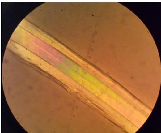
**Figure 4a):** DIC image of thin section of film (~200X); Seven layers are present, and from the above images, they were estimated to be 9 um (outer), 36 um (PP), 25 um (nylon), 6 um (PP), 25 um (nylon), 36 um (PP), and 9 um (outer).
