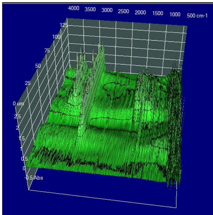
**Figure 5:** 3D Map of 5  $\mu\text{m}$  incremental FTIR scans across the 150  $\mu\text{m}$  thin film
