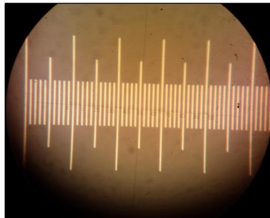
**4b)** Image of stage micrometer used to calibrate the reticle
