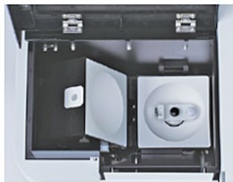
Figure 2: Top view of the integrating sphere (open position) within the sample compartment of an RF-6000, cuvette holder is in direct excitation position.
