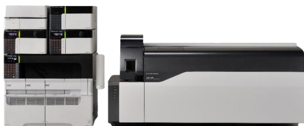
Liquid Chromatograph Mass Spectrometer LCMS-8050
