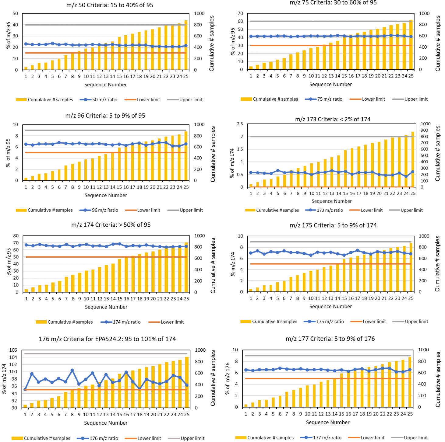
Figure 4: Evaluation of method 524 BFB Tune Criteria for 25 sequences over 7 weeks.
