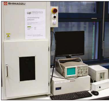
Fig. 1: Overview of the ultrasonic fatigue testing system USF-2000 by Shimadzu
