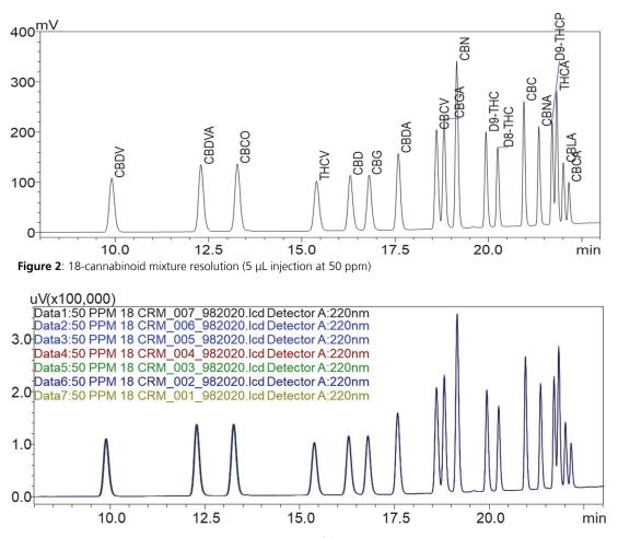
Figure 3: 18-cannabinoid mixture repeatability and overlay of seven-injections (5 µL injection at 50 ppm)
