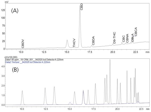
**Figure 9**: Tincture-1 profile (A); Tincture (blue trace) 1000x diluted vs. 85 ppm 18-Component Standard (black trace) (B). Results obtained at 5 µL injection volume.
