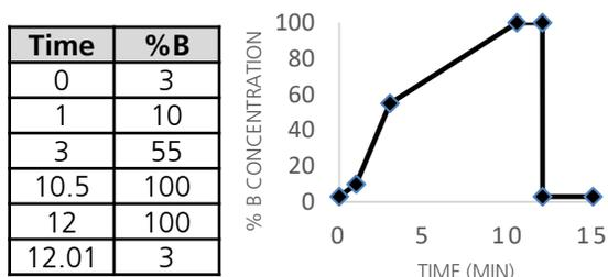
Figure 1: LC gradient Parameters
