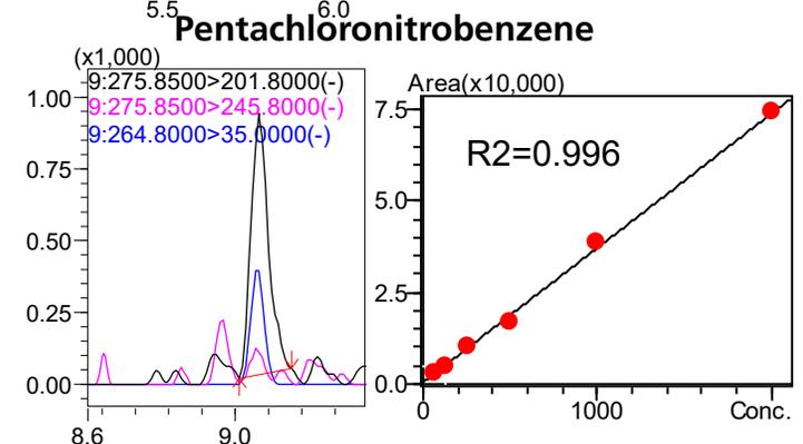
Figure 3: Calibration Curves and MS Chromatograms at 0.062ug/g in Cannabis Matrix for Ten Pesticides
