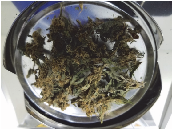
Figure 1: Picture of cannabis flower placed on the measurement pan of a MOC63u moisture analyzer
