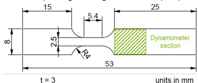
**Figure 2:** Specimen geometry
