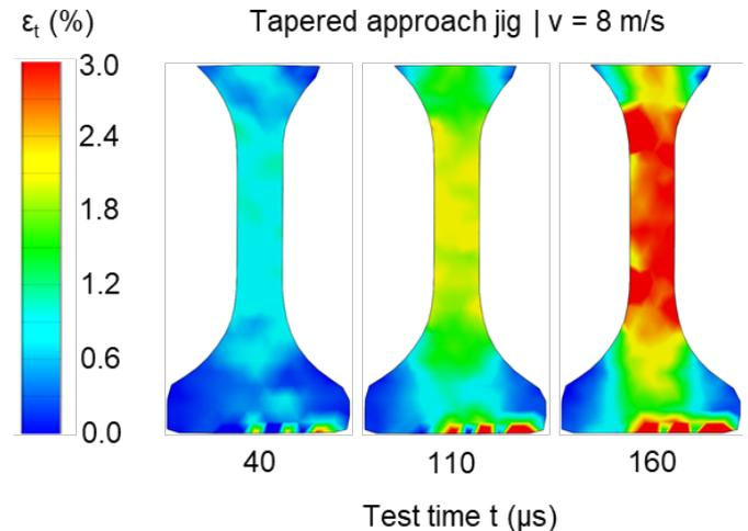
**Figure 7:** Specimen strain distribution at diff. test times
