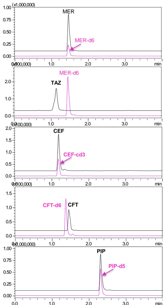
**Figure 3:** MRM chromatograms of five  $\beta$ -lactam antibiotics each (400 ng/mL) with internal standards in plasma on LCMS-8060
