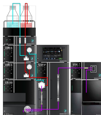
Figure 1: The delay column setup in the system for PFAS analysis.
