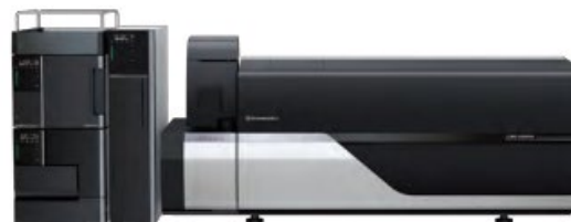
Figure 4: LCMS-8060NX configuration. The IonFocus design improves signal intensity with higher gas flows and higher effective temperatures. The probe position can be moved further from the MS inlet without losing signal intensity.
