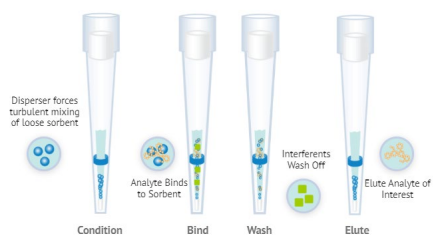
Figure 3: DPX Sample Preparation Procedure. Bind and wash solution: 50% methanol in water. Elution solution: acetonitrile.
