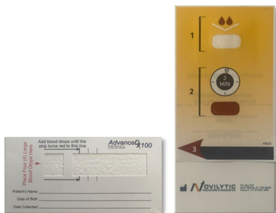
Figure 1: Two types of DBS cards. Left card produces ~30µL of serum; right card produces ~6µL serum.
