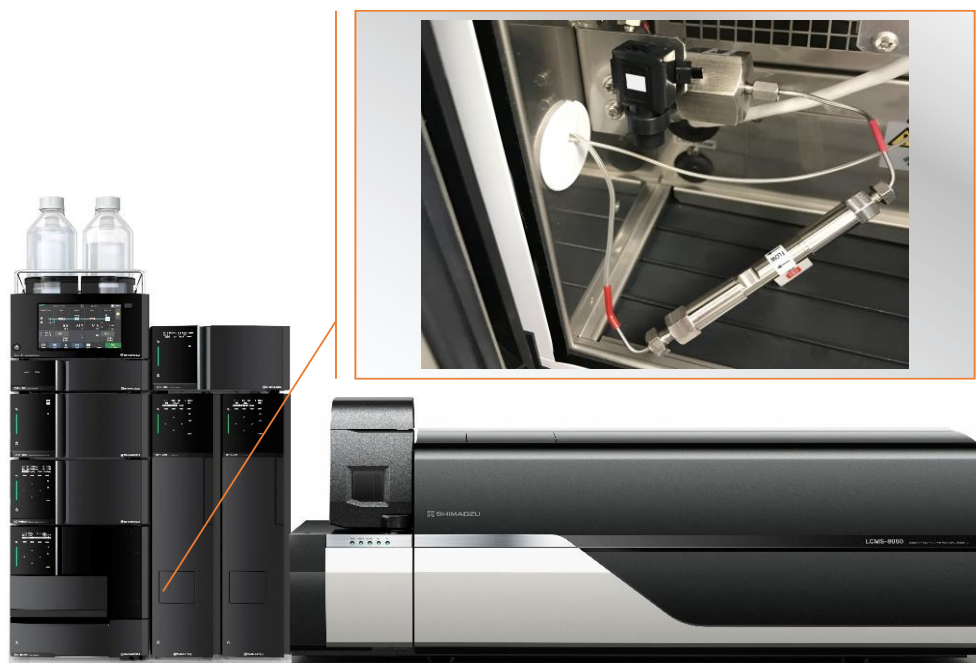
Figure 1: Installation/placement of a delay column for PFAS Analysis.
