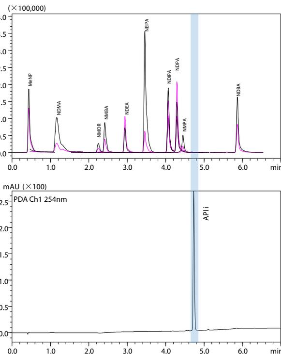
Fig. 4 Chromatograms for 0.1 ppm Spiked Sample
