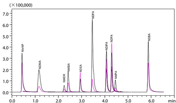
Fig. 2 Chromatogram of 10 ng/mL Mixed Nitrosamine Standard
