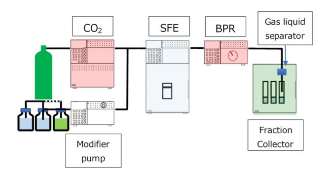
Figure 1. System Configuration of Nexera UC offline SFE system
