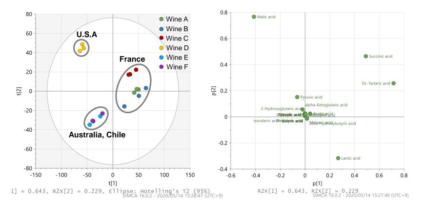
Figure 4 Score plot and loading plot in analysis of short chain fatty acids and organic acids
