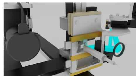
**Figure 1.** The IMScopeQT, a high-speed API-MALDI source connected to a QTOF mass spectrometer, was used to acquire data from mouse brains. A typical full mouse brain data set could be acquired in under 2 hours.
