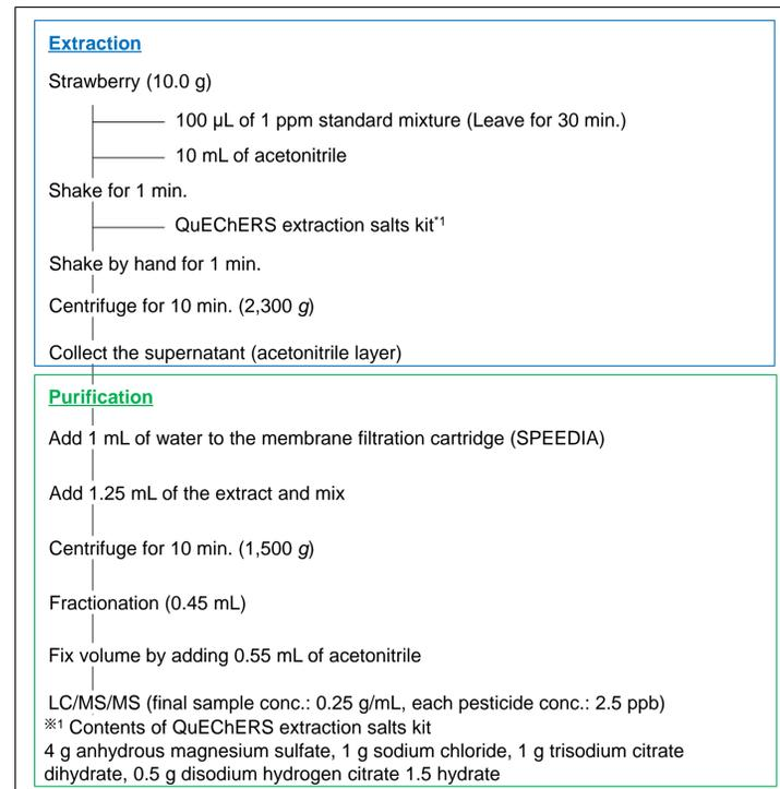
Fig. 1 Workflow for Sample Preparation
