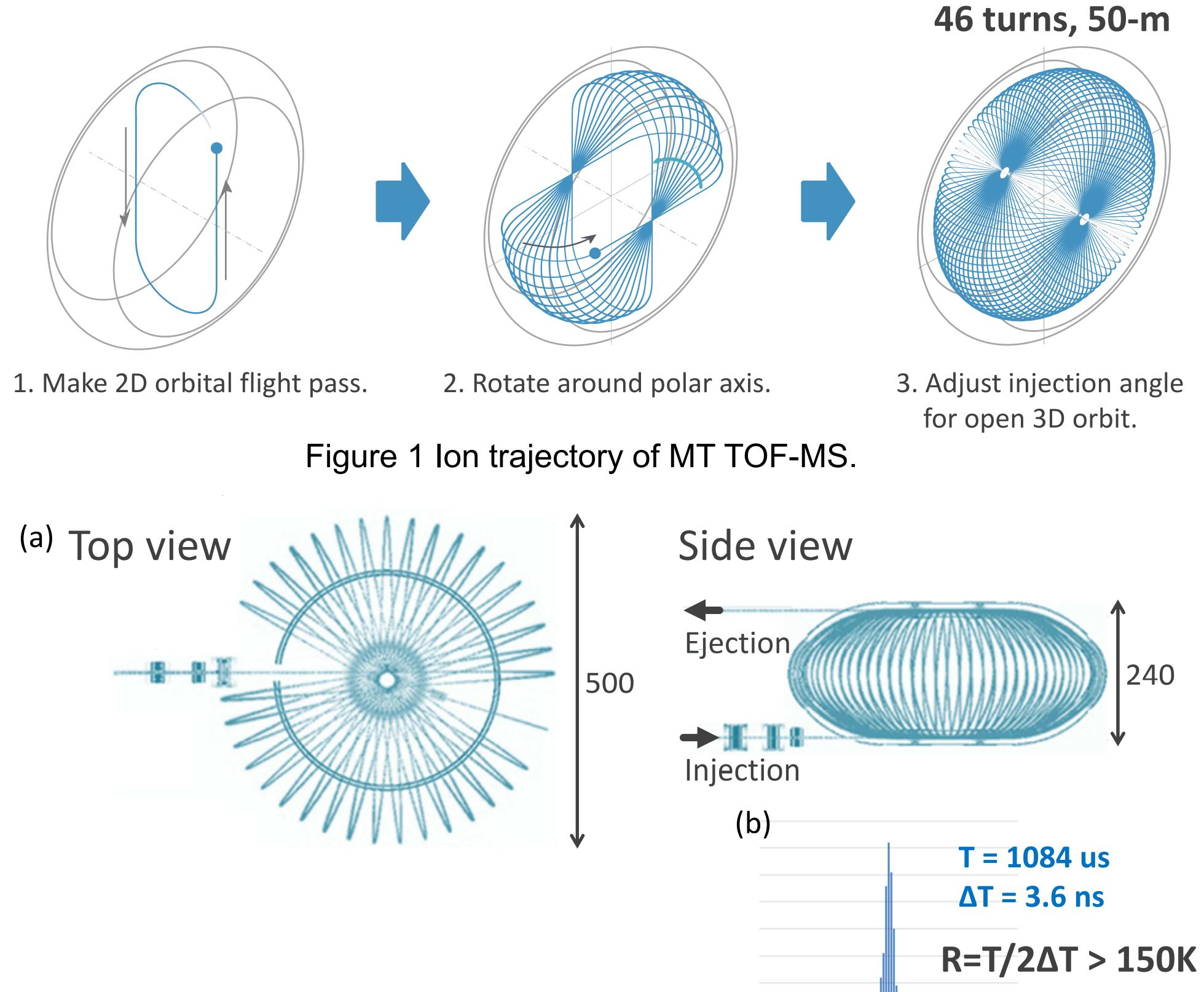
Figure 2 Simulated (a) ion trajectories and (b) TOF spectrum.
