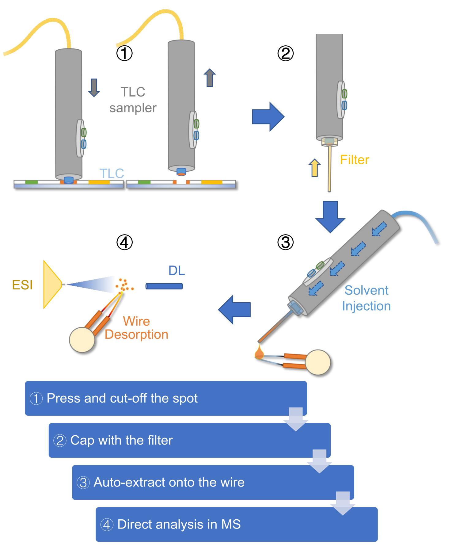
Figure 3. Operation procedure of TLC-MS analysis
