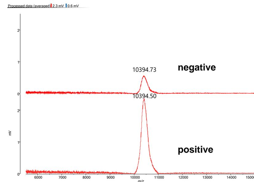
Figure 5. Direct analysis of RNA with 32 bases in Mg(NO<sub>3</sub>)<sub>2</sub> containing buffer without desalting in positive and negative ion mode.
