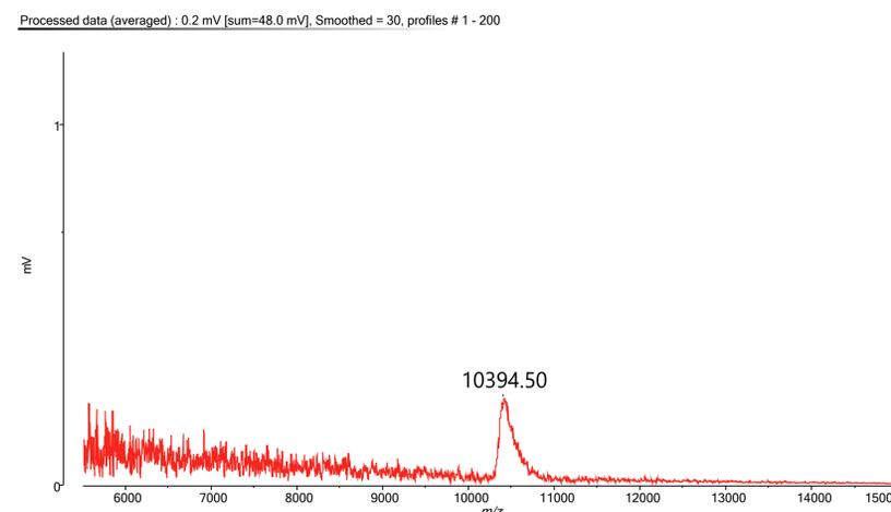
Figure 3. Analysis after desalting of RNA with 32 bases in MgCl<sub>2</sub> containing buffer.
