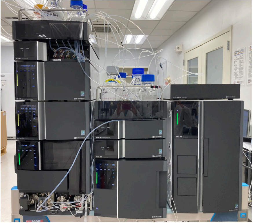
Fig. 2. Nexera Mikros trap and elute LC system with additional loading pump rinsing functionality.
