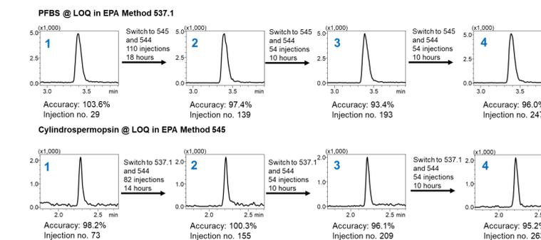
Figure 4: Mass chromatogram and quantitative accuracy of representative compounds before and after switching methods.
