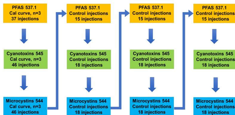
Figure 2: Batch structure designed to assess the performance and reliability of running three analytical methods on a single system.
