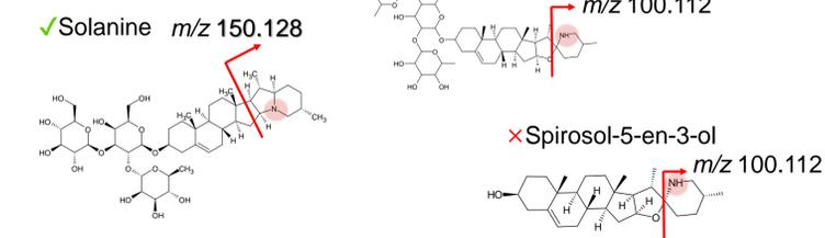
**Fig. 5** Structural analysis results by LabSolutions Insight Explore
