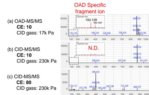
**Fig. 4** OAD or CID MS/MS mass spectra of [solanine+H]<sup>+</sup>
