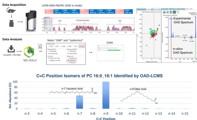
Fig. 3 Workflow of untargeted OAD-lipidomics using LC-MS.
