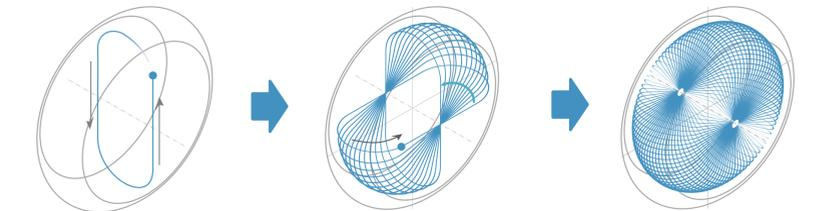
1. Make 2D orbital flight pass. 2. Rotate around polar axis. 3. Adjust injection angle for 3D orbit.
