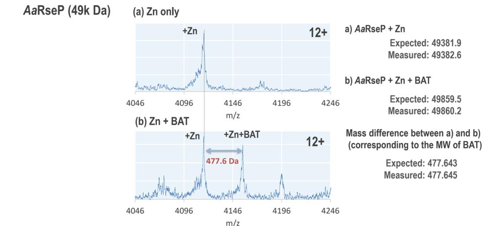
Figure 7. Native mass spectrum of AaRseP with LDAO ; bound to (a) Zn only ; (b) Zn and BAT
