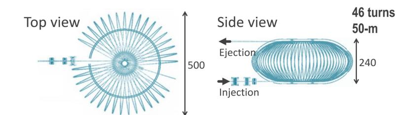
Figure 1. Ion trajectory of the multi-turn ion optical system
