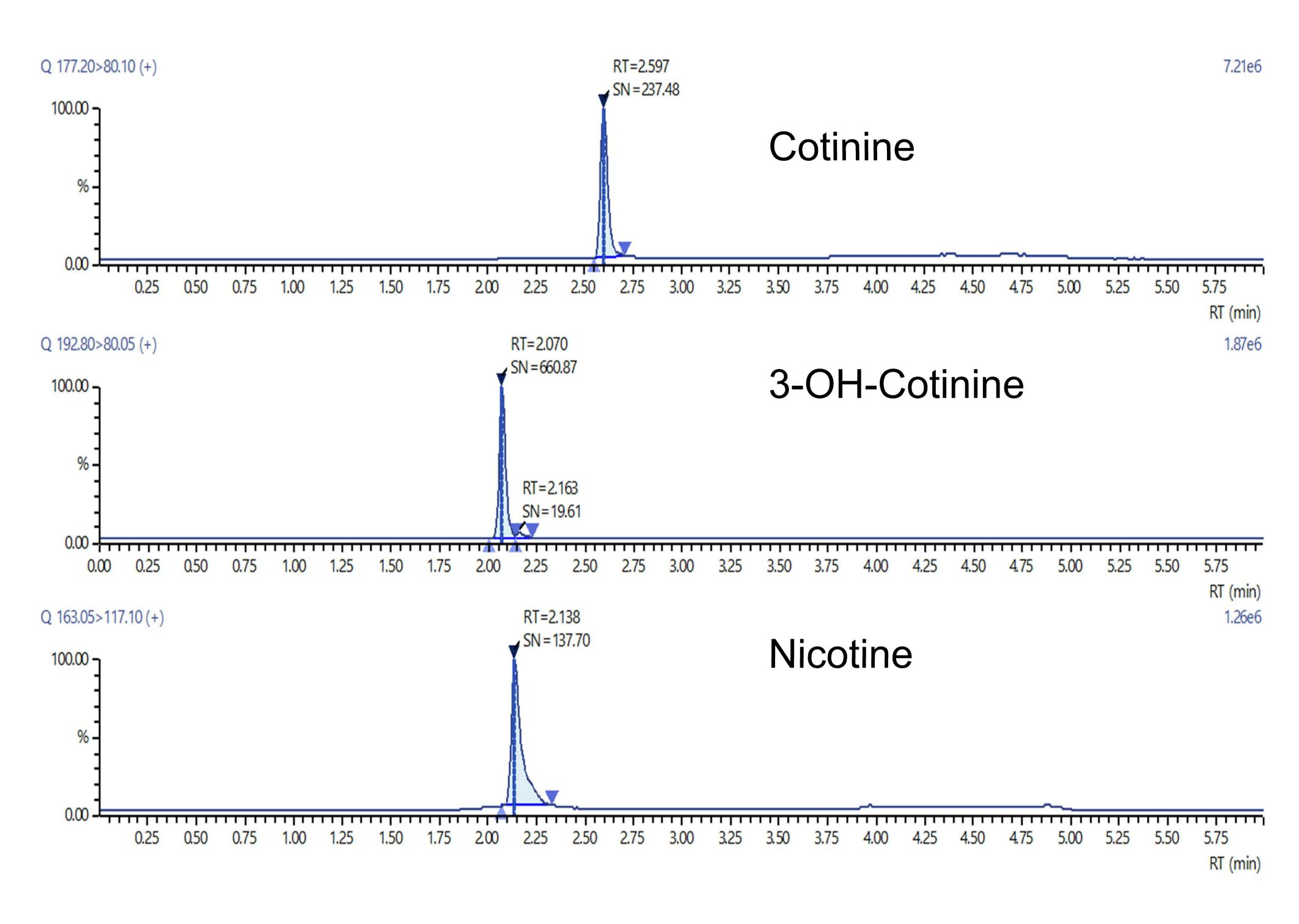
**Fig. 4** Example chromatogram of a Urine patient sample, containing Cotinine, 3-OH-Cotinine and Nicotine
