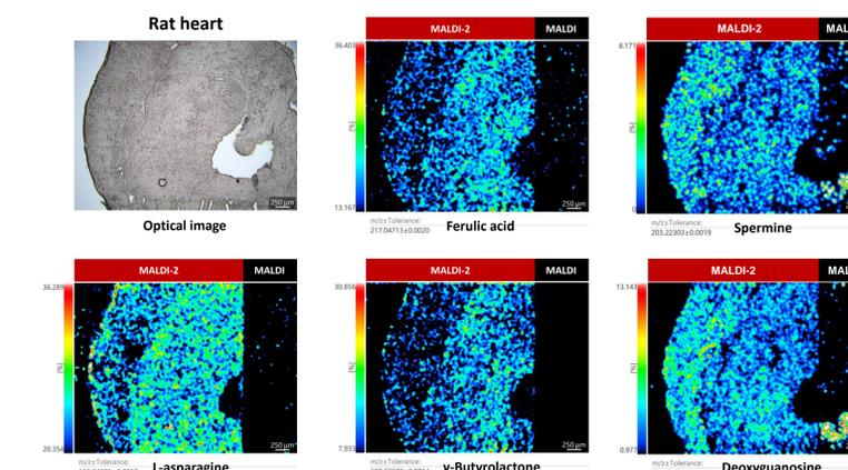
**Fig. 5** Optical image and MS images acquired from rat heart using iMScope with MALDI-2. Left half of each MS image was acquired with laser-2 ON, while right half was acquired with laser-2 OFF. Displayed metabolites: [ferulic acid + Na]<sup>+</sup>, [spermine + H]<sup>+</sup>, [L-asparagine + Na]<sup>+</sup>, [ $\gamma$ -butyrolactone + Na]<sup>+</sup>, [deoxyguanosine + H]<sup>+</sup>.
