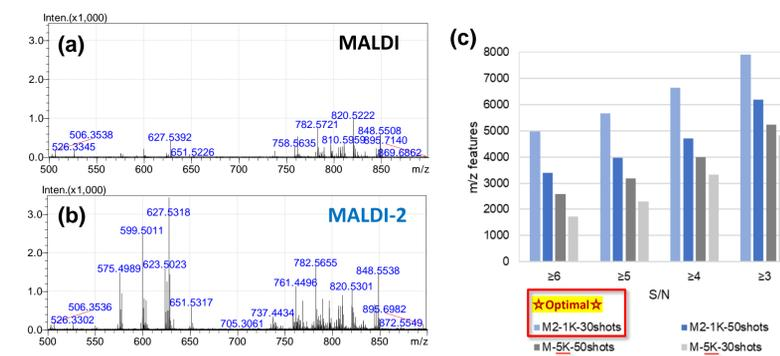
**Fig. 3** Averaged MS spectra of rat liver homogenate obtained with (a) MALDI and (b) MALDI-2. Laser repetition rate was 1 kHz. (c) Number of detected m/z features from averaged MS spectra obtained with 1-kHz MALDI-2 and 5-kHz MALDI. Mass range: 500~900 m/z. Optimal parameters: M2 (MALDI-2) – 1K (laser repetition rate) – 30 shots (per pixel).
