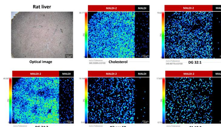
**Fig. 4** Optical image and MS images acquired from rat liver using iMScope with MALDI-2. Left half of each MS image was acquired with laser-2 ON, while right half was acquired with laser-2 OFF. Displayed metabolites: [cholesterol - H<sub>2</sub>O + H]<sup>+</sup>, [DG 32:1 - H<sub>2</sub>O + H]<sup>+</sup>, [DG 34:2 - H<sub>2</sub>O + H]<sup>+</sup>, [ribose 5P + H]<sup>+</sup>, [FA 18:3 + H]<sup>+</sup>.
