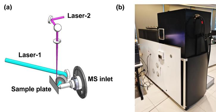
**Fig. 1** (a) Illustration of the second laser for post ionization. (b) Photo of the upgraded iMScope QT with MALDI-2.
