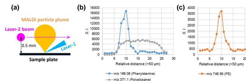
**Fig. 2** (a) Illustration of the scanning of the position of laser-2 beam. (b) Phenylalanine sample. Polysiloxane ((C<sub>2</sub>H<sub>6</sub>SiO)<sub>5</sub>, m/z = 371.10) from ambient air was also ionized by laser-2. (c) PE (18:0-18:1) sample.
