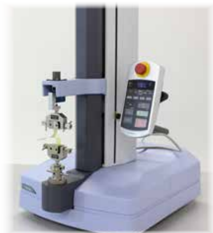
Shimadzu EZ-X Universal Tester tearing paper
