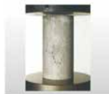
Compression testing of explosion proof cement
