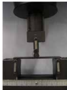
3-point bending on a Shimadzu Universal Testing Machine
