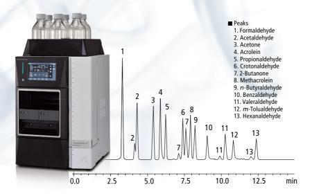
The i-Series integrated LC system offers ultimate performance for routine QA/QC analysis in a very compact format. Reliable quantitative data is provided through high-speed analysis with minimized environmental impact, easy maintenance and ease of use through touch panel control, chromatogram monitor and easy-batch function. The i-Series is a powerful tool for the determination of nicotine, caffeine, aldehydes or nitrosamines in e-liquids, even for novices in instrumental analysis.
