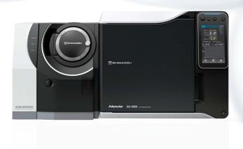
The combination of the GCMS-QP2020 NX single quadrupole mass spectrometer with the FID-2010 Plus detector allows a very simple and robust determination of nicotine concentration (by flame ionization), identification of CAS# and IUPAC-name (by mass spectrometry), and quantitation of many flavor compounds in e-liquids.
